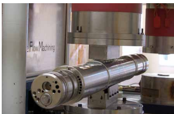
Abrasive flow deburring and ultrasonic cleaning ensures burr-free internal features
