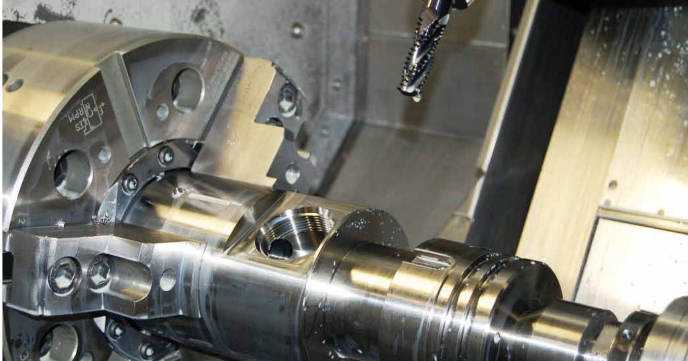
5-axis, single-cycle turn-milling on Mazak Integrex
